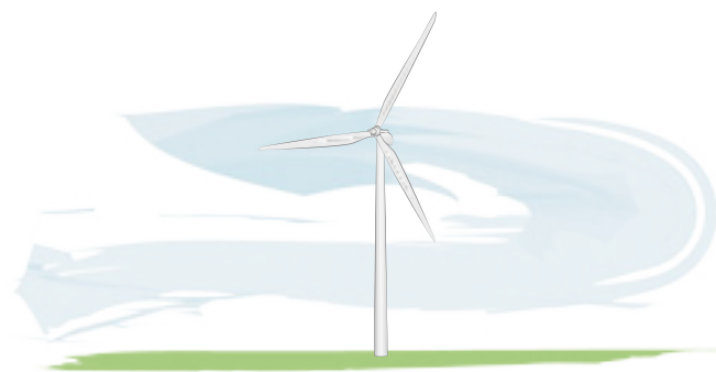
Horizontal axis wind turbine
