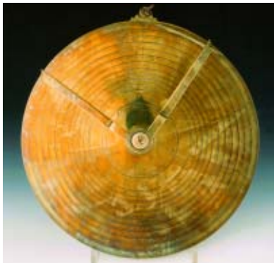
An example of the first slide rule, the 'Circles of Proportion', designed by the eminent mathematician William Oughtred in the 1630s and made by Elias Allen in 1648.
